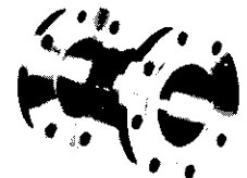
MODEL 50MY15 All stainless steel welded unit with fused matrix. Differential pressure connections are 1/4" NPT. Line connections are Series 15 flanges. Max. design: 150 PSIG and 150° F.
