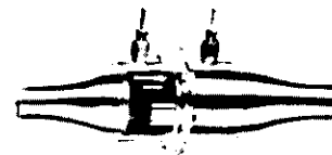
MODEL 50MC2 This flow element is for low pressure applications. Differential pressure connections are 1/4" NPT. Designed for use with hose for line connections at inlet and outlet. To include inlet filter, add suffix "F". Max. design: 20 PSIG and 150° F.
